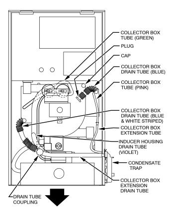
Fig. 8—Downflow Tube Configuration (Right-Hand Trap Installation)
